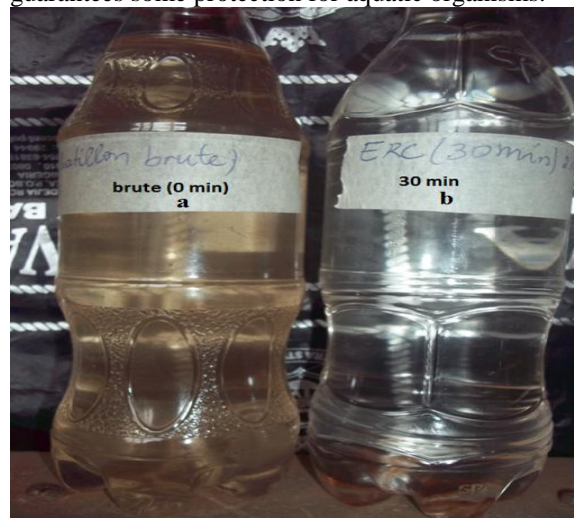
Figure 3: Water samples from river Choumlou (a): raw untreated sample (b): sample treated at 30 mins by the Gliding arc plasma
